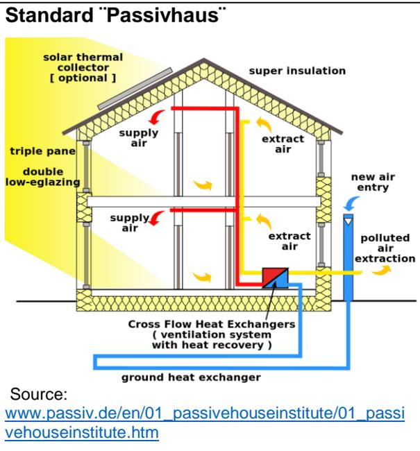
In Passivhaus buildings, the cost savings from dispensing with the conventional heating system can be used to fund the upgrade of the building envelope and the heat recovery ventilation system. With careful design and increasing competition in the supply of the specifically designed Passivhaus building products, in Germany it is now possible to construct buildings for the same cost as those built to normal German building standards.
